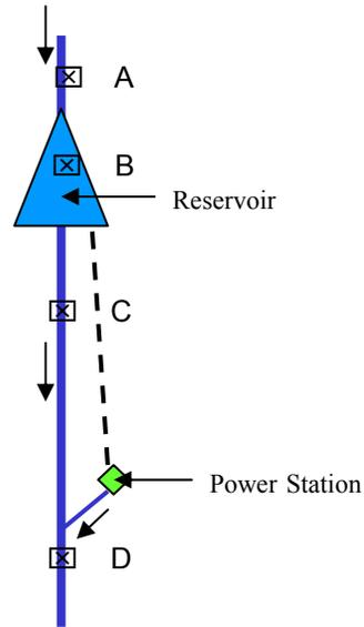
Run-of-river dam and power station with dewatered reach between dam and power station. Sampling locations include: Upstream of reservoir (A), within reservoir (B), within dewatered reach (C), and downstream from tailrace confluence with river (D).
