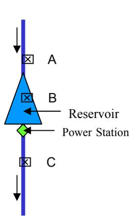
Run-of-river dam and power station. Sampling locations include: upstream from reservoir (A), within reservoir (B) and downstream (C) from power station.
