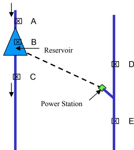
Run-of-river dam and power station with interbasin diversion. Sampling locations include: upstream from reservoir (A), within reservoir (B), downstream from dam (C), upstream from tailrace (D) and downstream from tailrace (E).
