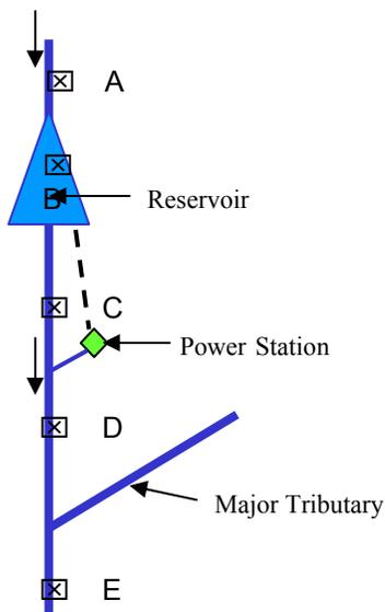
Run-of-river dam and power station with dewatered reach and major tributary downstream of tailrace. Sampling locations include: upstream of reservoir (A), within reservoir (B), within dewatered reach (C), downstream from tailrace (D), and downstream from tributary (E).
